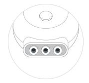
Insert the sensors jack plug into the transmitter.
