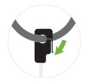
Place the sensors around the live feed cable of your electrical panel.
