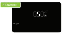
By default the carbon emissions ratio is 0.50 kgCO₂. Use the ◀ BACK/DOWN and ▶ NEXT/UP buttons to increase or decrease the value. Tap ☐ MODE/SET button to confirm and move onto the calibration set up.
