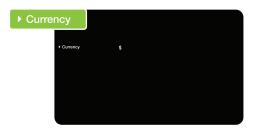
Select the currency using the **4 BACK/DOWN** and **> NEXT/UP** buttons. The default currency will be \$. Tap the **MODE/SET** button to confirm and to move onto tariff selection set up.
