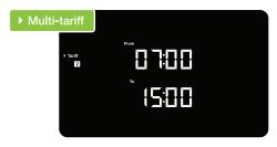
You can select up to 4 different tariffs. Tap the ♠ MODE/SET button to set up tariff 2, use the ◀ BACK/DOWN and ▶ NEXT/UP to configure the time period and tap the ♠ MODE/SET button to move to the tariff pricing.
