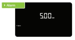
The high usage alert will be displayed if you go over your set maximum power consumption target. Use the ◆BACK/DOWN and ▶ NEXT/UP buttons to set the value. Tap the ♣ MODE/SET button to confirm and move onto footprint set up.
