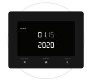
The first time that you power on the monitor, the screen will light up and ask you to enter the correct day, month, year and time. Use the ◀ BACK/DOWN and ▶ NEXT/UP buttons to change values and the ♣ MODE/SET button to save.
