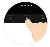
Enter in the settings menu and complete the on-screen steps to set up your device. In the setting mode use the **\BACK/DOWN** and **\DEXT/UP** buttons to increase or decrease the digit numbers, press the **\Text{\DEMODE/SET}** button to confirm and continue to the next setting.
