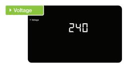
Adjust the voltage using the ◆BACK/DOWN and ▶ NEXT/UP buttons. Tap the MODE/SET button to confirm and to move onto currency selection set up.
